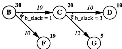
Figure 3: An Example for Calculating  $max\_delay\_to\_sink$  and  $branch\_slack$
