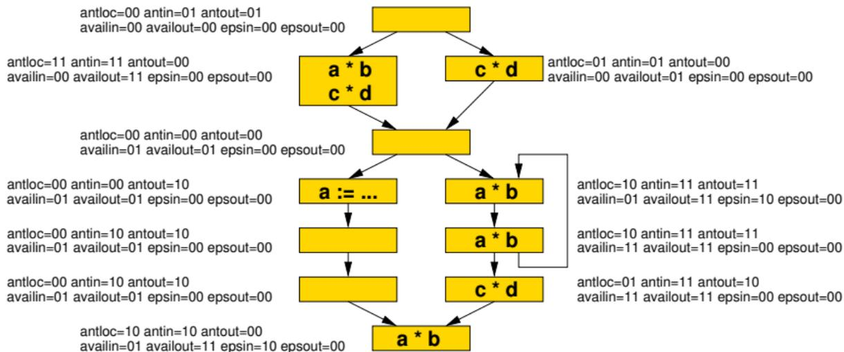
$$\begin{aligned} \text{epsin}_e(b) &= (\sum_p (\text{availout}_e(p) + \text{epsout}_e(p))) \cdot \text{antin}_e(b) \cdot \neg \text{availin}_e(b) \\ \text{epsout}_e(b) &= \text{epsin}_e(b) \cdot \neg \text{antloc}_e(b) \end{aligned}$$
