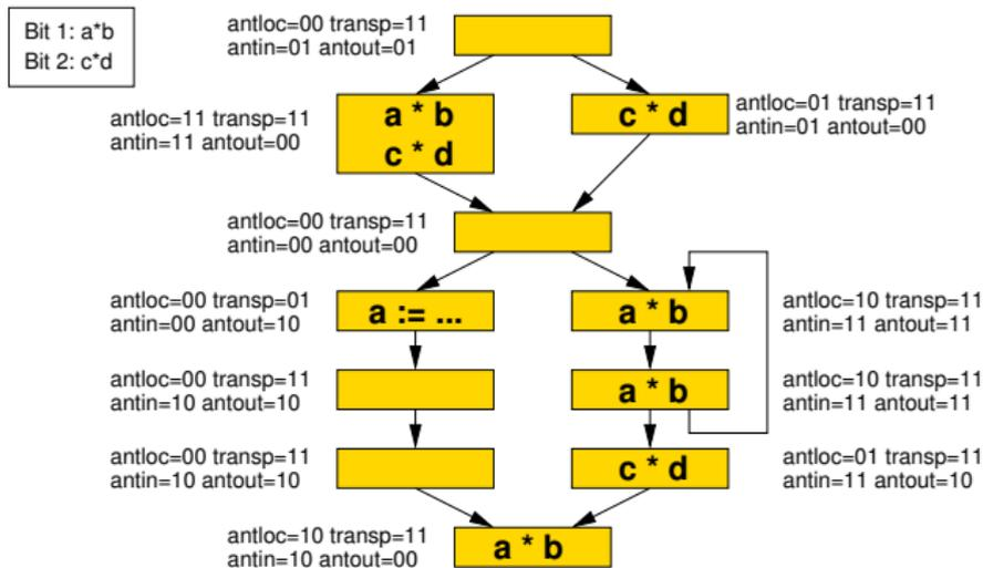
$$\text{antin}_e(b) = \text{antout}_e(b) \cdot \text{transp}_e(b) + \text{antloc}_e(b)$$
