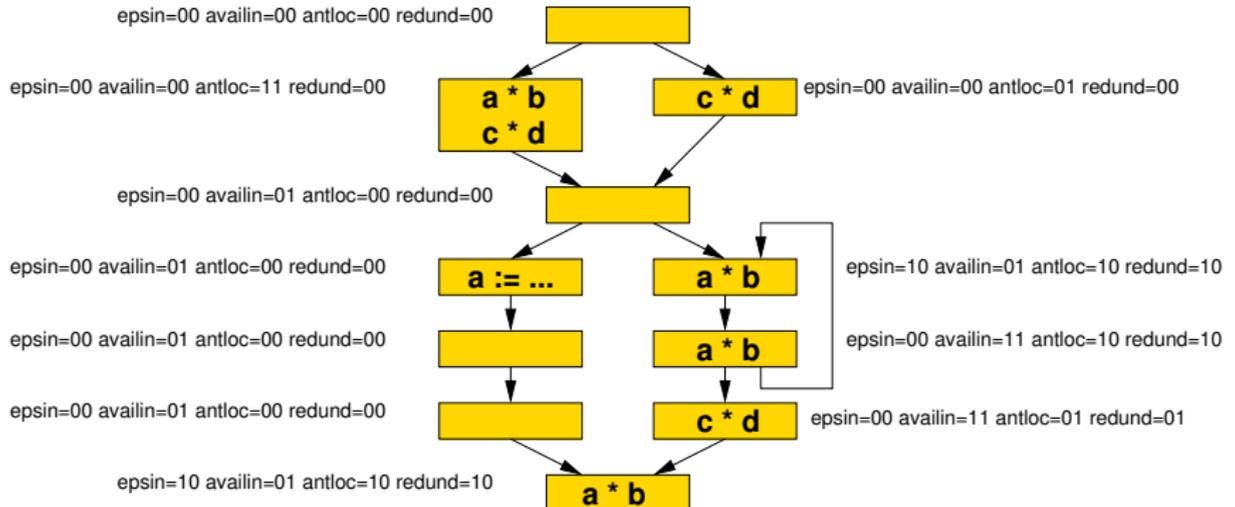
$$\text{redund}_e(b) = (\text{epsin}_e(b) + \text{availin}_e(b)) \cdot \text{antloc}_e(b)$$
