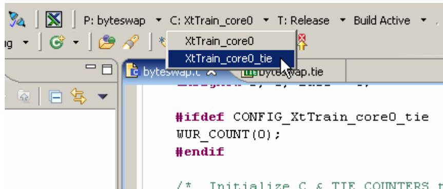
We need to tell Xplorer that we want to build the software project **byteswap** for the core **XtTrain\_core0\_tie** in the new system.
