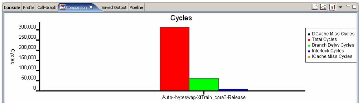
The chart shows the data cache miss cycles, total cycles taken by the code, branch delay cycles, interlock cycles and instruction cache miss cycles.
