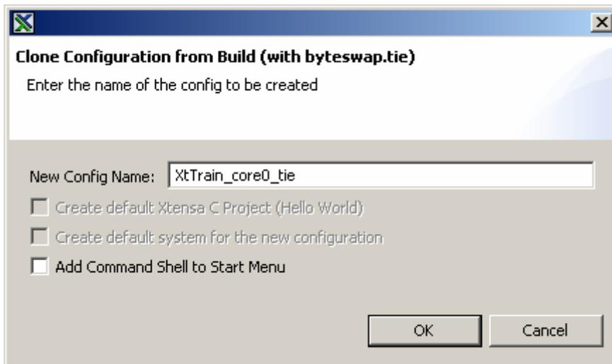
The name of the original processor configuration is **XtTrain\_core0**. The clone processor configuration name is **XtTrain\_core0\_tie**. These two processor configurations are shown under **XtTrain\_core0-params** in the System Overview View's Configurations folder.
