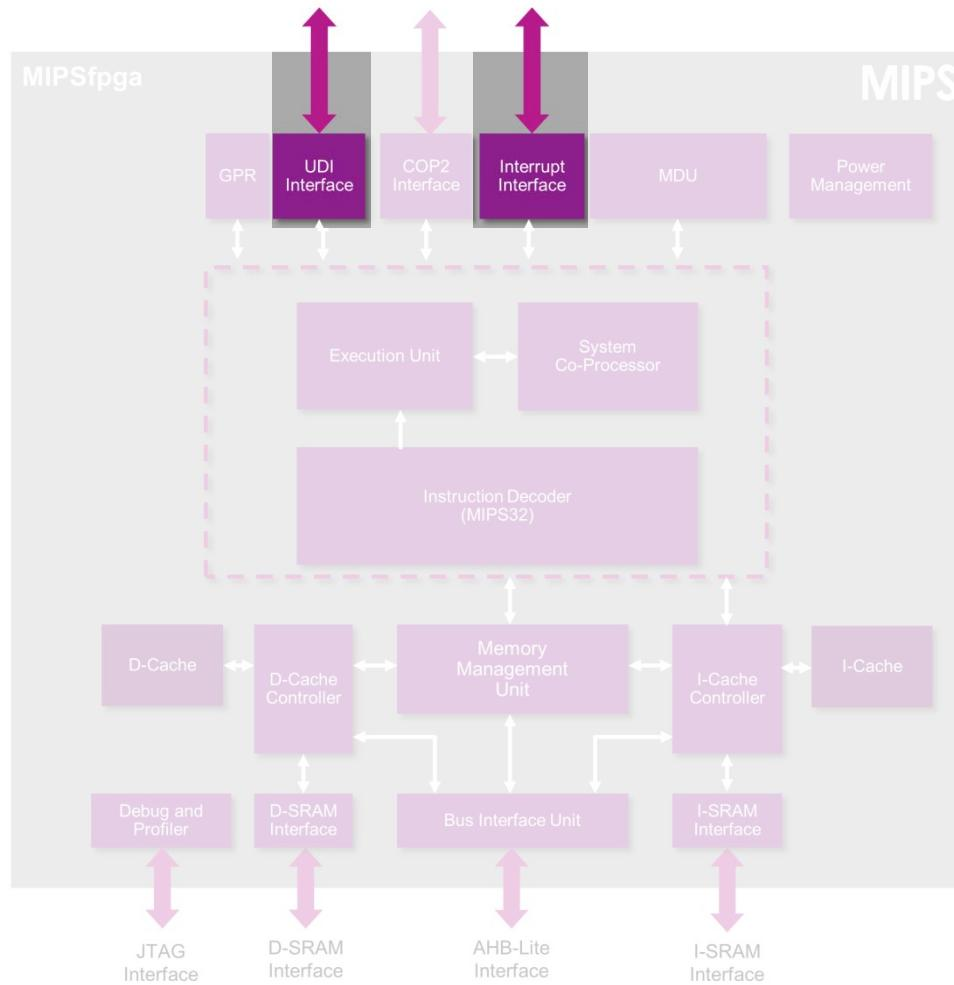
**Interrupt Interface:** used for hardware interrupts
