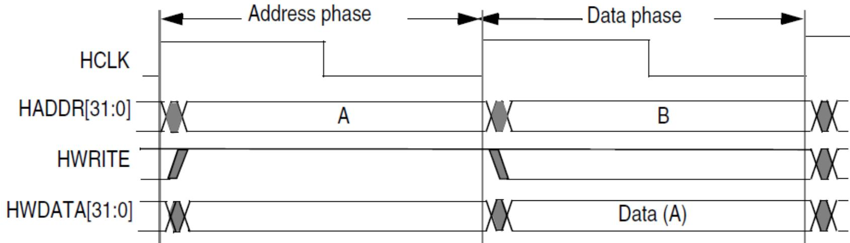
**Cycle 1: Address and Write Enable (HADDR & HWRITE)**
