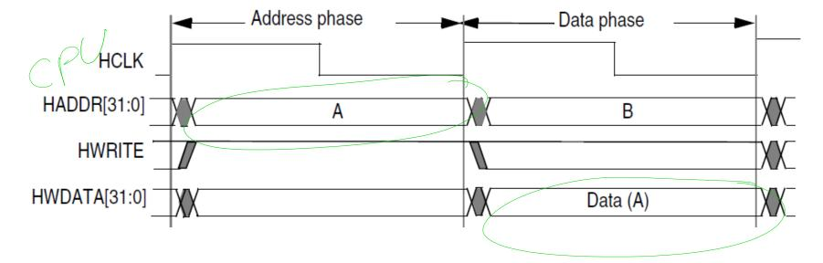
Cycle 1: Address and Write Enable (HADDR & HWRITE) Cycle 2: Write Data (HWDATA)
