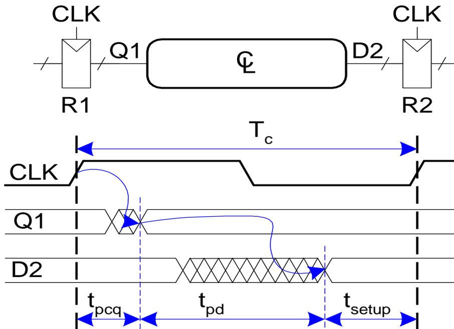
$$T_c \geq t_{pcq} + t_{pd} + t_{\text{setup}}$$
