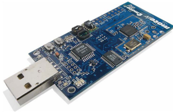
Figure 1.1: Common wireless sensor network platform Tmote Sky. This platform provides a TI MSP430F1611 microcontroller, 48 kbyte Flash and a 250 kbps wireless transceiver. Furthermore, it features various possibilities to access sensors. With as little as 15.3\mu\text{W} power consumption in sleep mode this device can operate without human interaction for long times. Source: http://www.snm.ethz.ch/snmwiki/pub/uploads/Projects/tmote_sky_small.jpg
