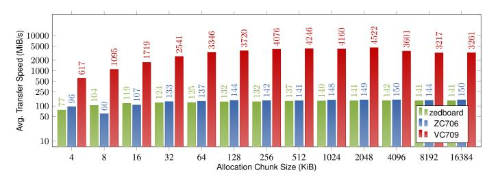
Fig. 4: Average bidirectional transfer rates between FPGA and host (i.e., user application memory) in MiB/s.
