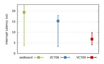
Fig. 5: Interrupt latencies: measured round-trip time (max/avg/min) between a hardware kernel signaling an interrupt and then receiving an acknowledgement from the host.
