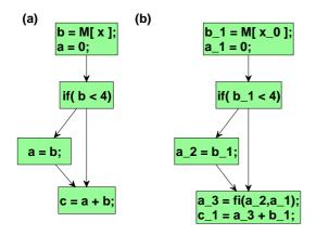
Fig. 2: CFG (a) and CFG in SSA-Form (b)
