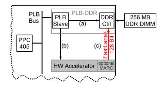
Fig. 10. FastLane+: Attaching HA directly to DDR controller
