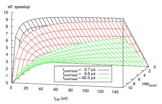
Fig. 18. Effective speedup as function of HA execution time and raw HW acceleration factor for different latencies
