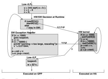
Fig. 4. Example in the Nimble execution model
