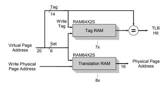
Fig. 17. PHASE/V MMU system: Tag- and translation RAM
