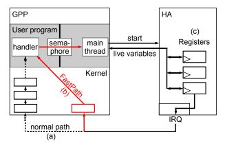
Fig. 8. FastPath: Low-latency SW calls and live variable transfers
