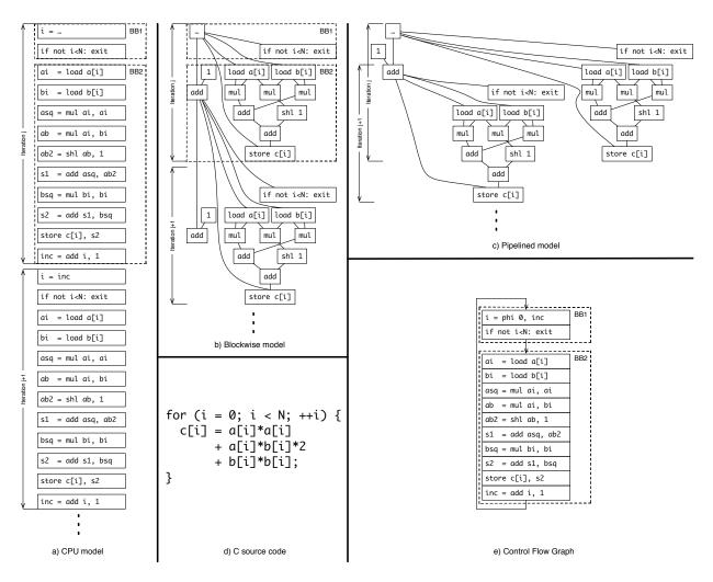
Fig. 1. Execution of two subsequent iterations of an example loop, according the presented execution models
