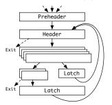
Fig. 2. Basic blocks of interest in a loop
