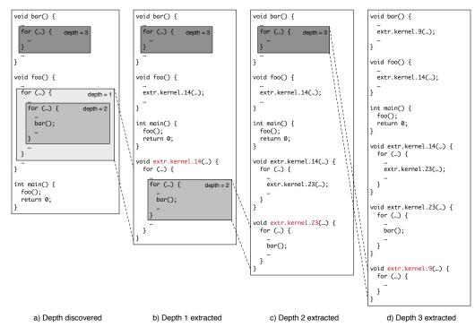
Fig. 3. Kernel depth and successive extraction
