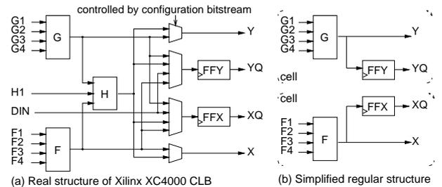
**Fig. 5:** Real and simplified structures for XC4000 CLBs
