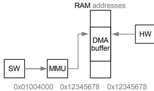
Figure 6: HW and SW addressing of DMA memory
