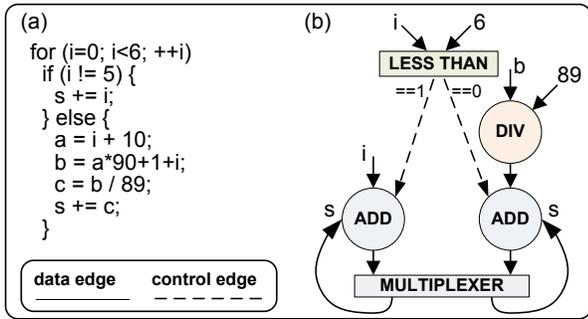
**Fig. 6.** Mismatched length in converging paths: (a) C source; (b) hardware.
