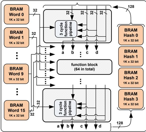
Fig. 7. MD5 Modlib HW Kernel Architecture
