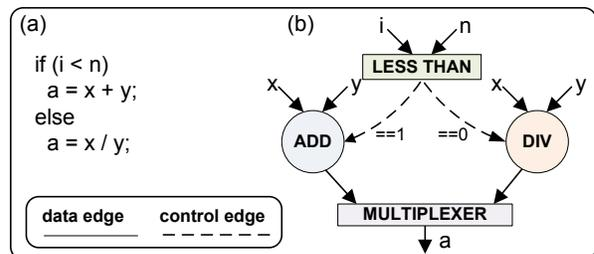
**Fig. 1.** Speculative execution of alternative branches of an if: (a) C source; (b) speculative predicated data flow.
