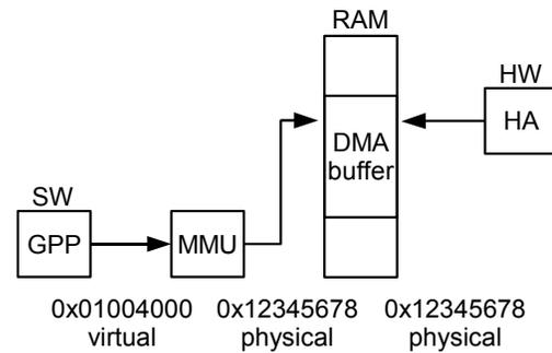
Fig. 12. Hardware and software addressing of memory
