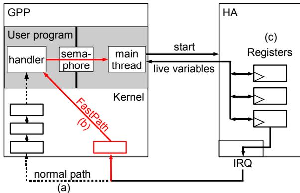
Fig. 8. FastPath: Low-latency SW calls and live variable transfers
