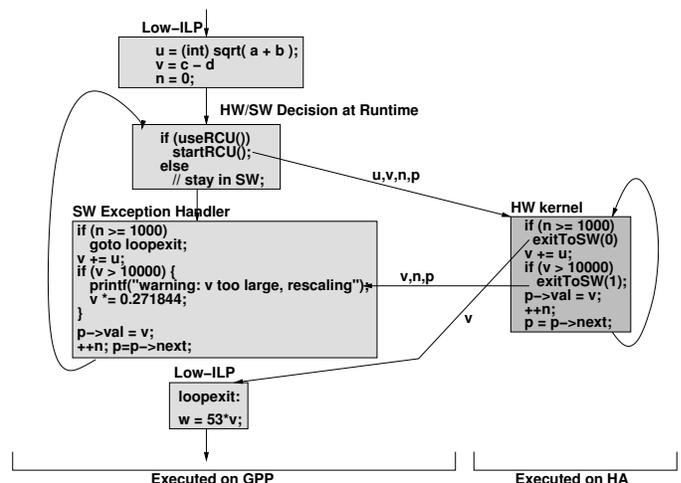
Fig. 4. Example in the Nimble execution model
