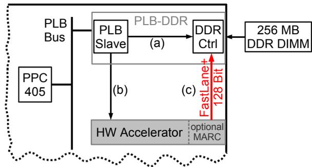
Fig. 10. FastLane+: Attaching HA directly to DDR controller
