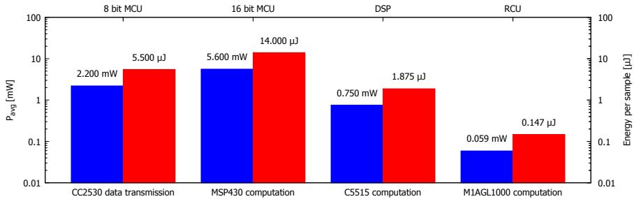
**Fig. 5.** Comparison of MCU- and RCU-based FIR implementations
