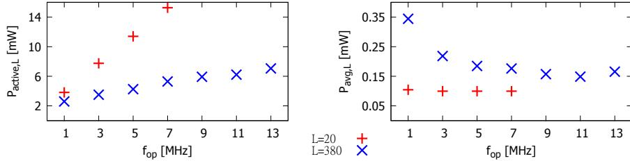
**Fig. 3.** Measured active and average M1AGL1000 power draw; computation of duty cycle for 384-FIR at different operating clock frequencies
