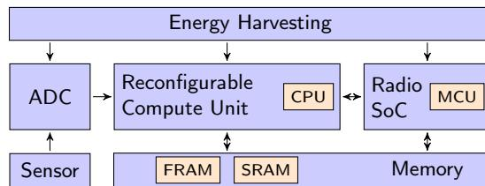
**Fig. 1.** Simplified overview of the *HaLoMote* platform
