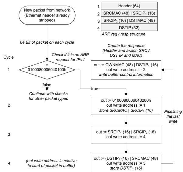
Figure 3. Zero-cycle overhead ARP response generation
