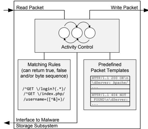
Figure 4. Schematic overview of the VEH components
