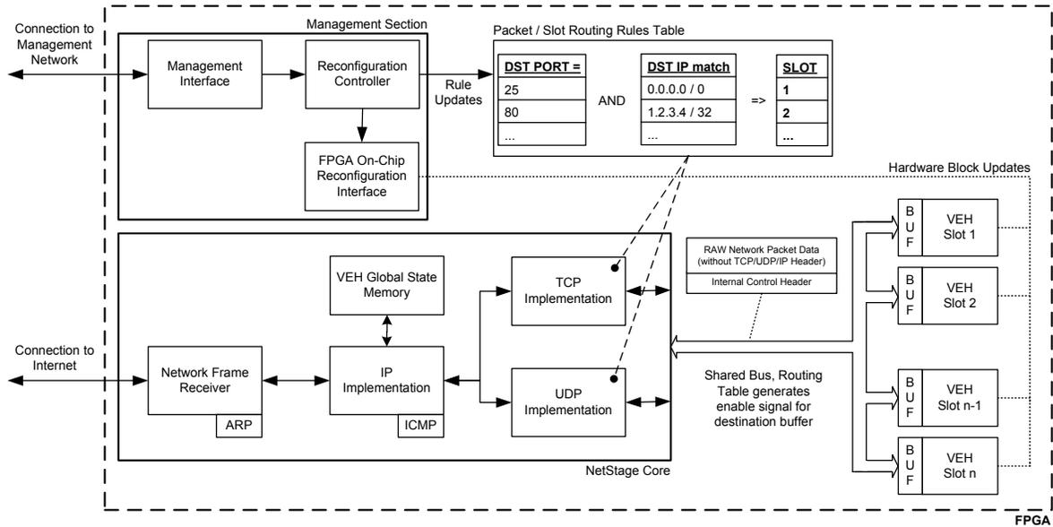
Figure 2. Core architecture of the malware collection network platform
