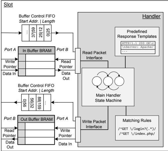
Figure 2: Slot wrapper and Handler architecture
