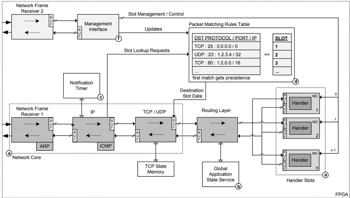
Figure 1: Core architecture of NetStage
