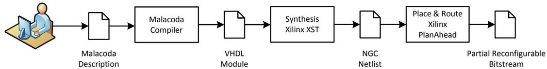
Figure 4: Tool flow for generating hardware from Malacoda programs
