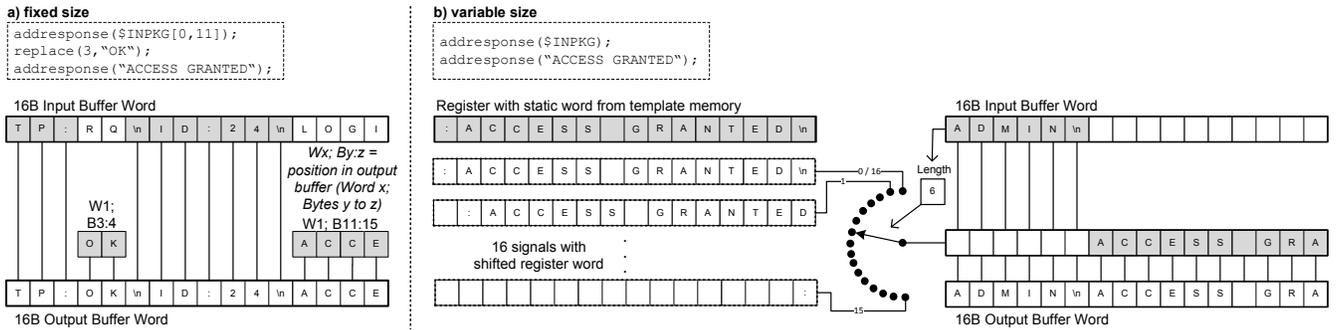
Figure 6: Construction of output packet for fixed and variable-sized response
