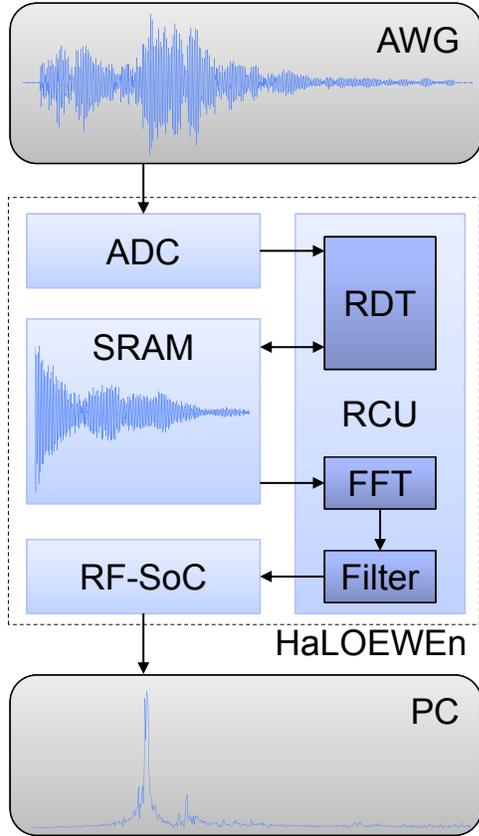
**Fig. 1.** Demonstration setup: Generation, aggregation and analysis of structural vibration data
