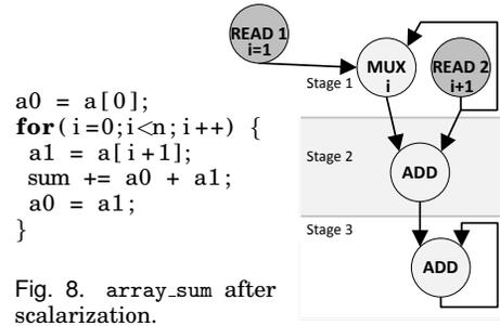
Fig. 8. array\_sum after scalarization.
