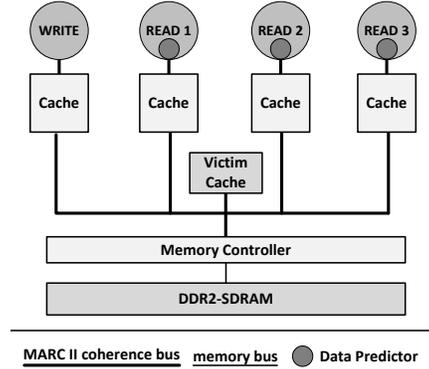
Fig. 4. MARC II memory system extended with read value speculation and victim cache
