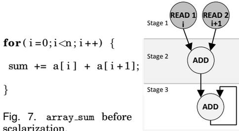
Fig. 7. array\_sum before scalarization.
