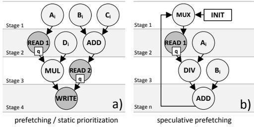
Fig. 5. Interaction of speculation with prefetching.
