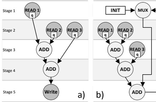
Fig. 6. Scenarios for prefetching interfering with rapid replays.
