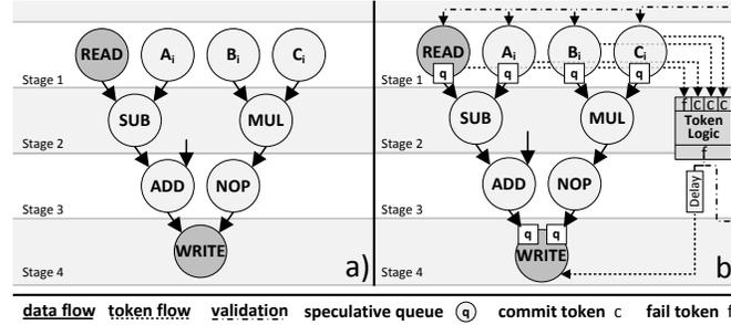
Fig. 1. Datapath and speculation token processing.
