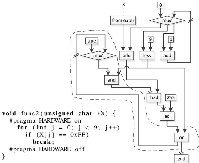
Fig. 11. Sample code and CDFG of a `for` loop requiring guard conditions.
