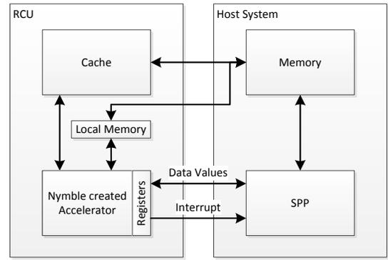
Fig. 1. Adaptive Computing System (ACS)
