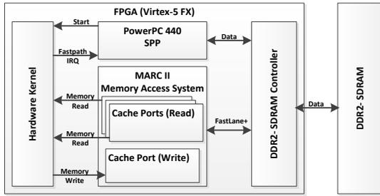
Fig. 2. ACS based on the Xilinx ML507 Virtex 5 FX FPGA Board
