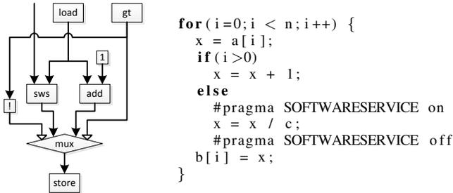
Fig. 8. Software service for resolving the CFG disadvantage of Fig. 5
