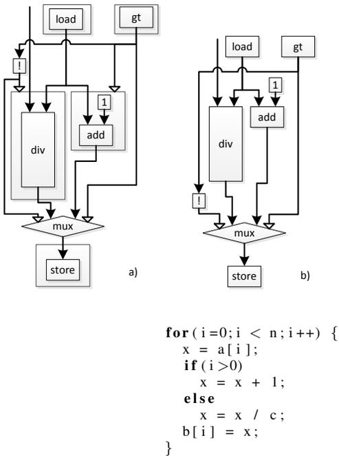
Fig. 5. Separate DFGs vs. single CDFG: Advantage DFGs
