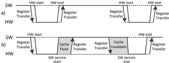
Fig. 7. Accelerator invocation protocol (solid line signifies control, dotted line is stored state while suspended)
