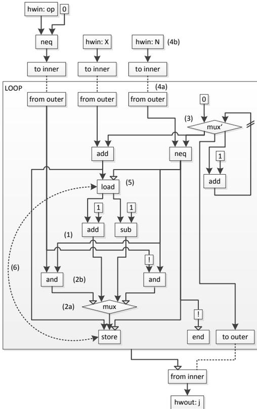
Fig. 10. CDFG of the hardware function from Fig. 6
