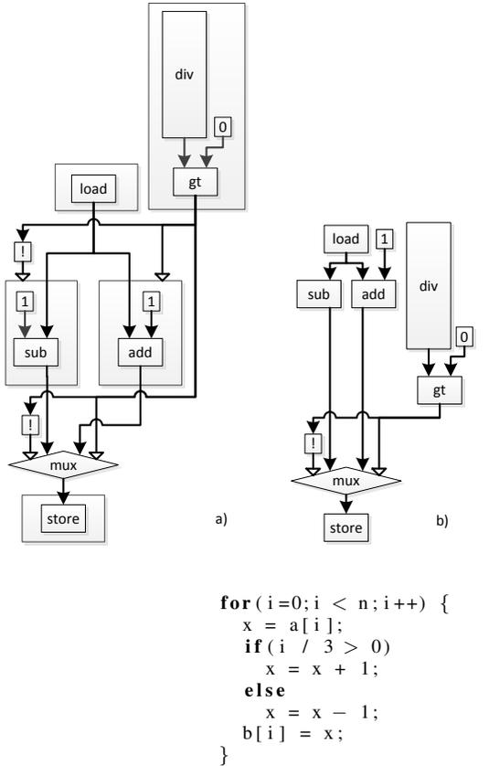
Fig. 4. Separate DFGs vs. single CDFG: Advantage CDFG
