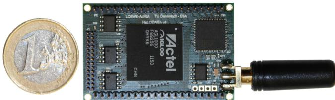
Fig. 3. Current implementation of the HaLoMote architecture
