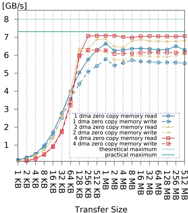
Figure 7: Throughput using multiple DMA engines
