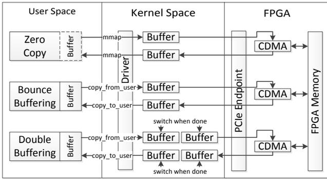
Figure 5: Driver transfer methods
