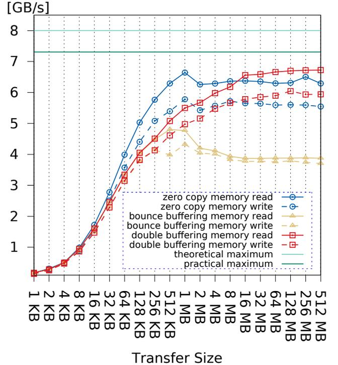
Figure 6: Throughput using single DMA engine
