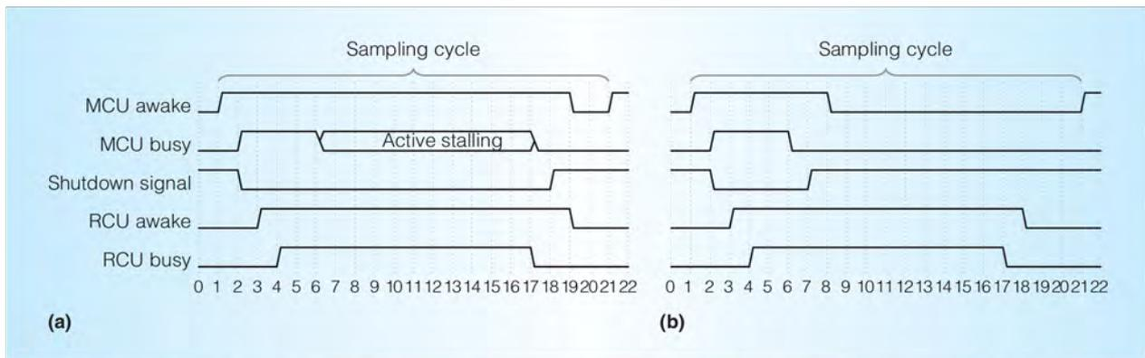
Figure 3. Scheduling of dynamic power management between the MCU and the RCU: (a) stalling the MCU and (b) delayed Flash-Freeze.
