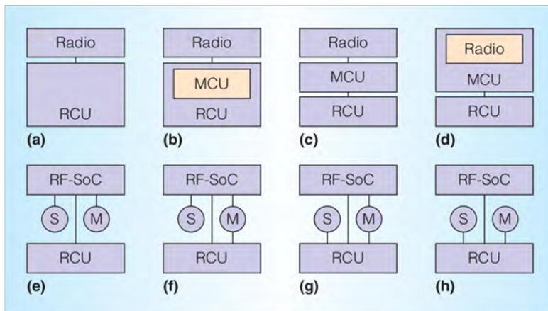
Figure 1. Design options for (a–d) the processing and communication architecture and (e–h) the attachment of sensors (S) and memories (M) to the computing units. (MCU: microcontroller; RCU: reconfigurable computing unit; RF-SoC: radio frequency system on chip.)
