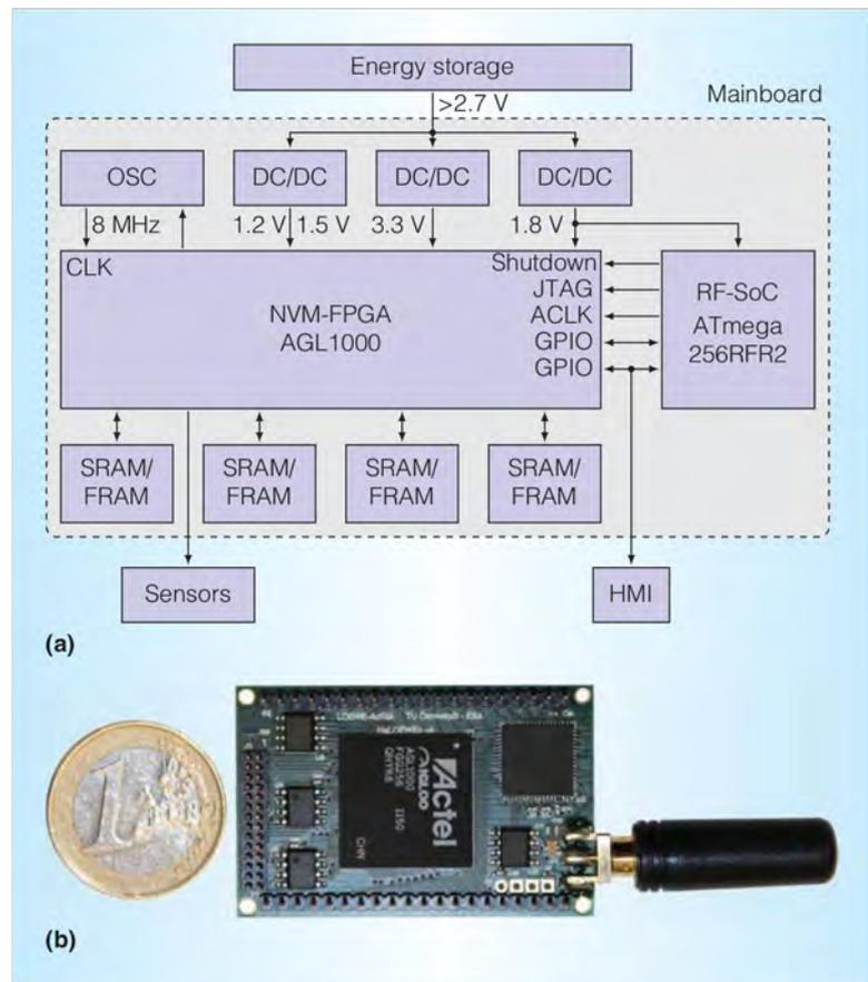
Figure 2. Implementation of Hardware-Accelerated Low-Power Mote (HaLoMote): (a) schematic and (b) 46 mm × 30 mm printed circuit board. (ACLK: auxiliary clock; FRAM: ferroelectric RAM; GPIO: general-purpose I/O; HMI: human-machine interface; JTAG: Joint Test Action Group; NVM-FPGA: nonvolatile memory field-programmable gate array; OSC: oscillator; SRAM: static RAM.)
