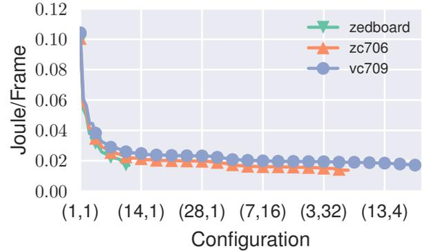
Figure 13: Energy consumed by different configurations of VGA-resolution accelerators when achieving 30 fps
