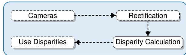
Figure 1: Typical stereo vision system. This paper focuses on the disparity calculation step.
