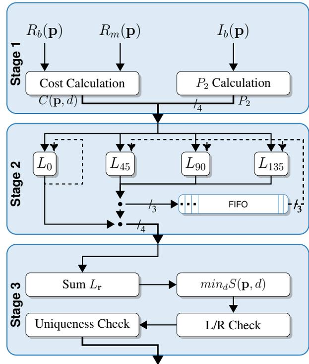
Figure 3: Base architecture for SGM. Stage 1 produces the per-pixel costs and  $P_2$  penalty values. Stage 2 calculates the path costs, using the outputs of the previous stage as well as prior paths costs stored in a stage-internal buffer. Stage 3 computes the disparities from the path costs.
