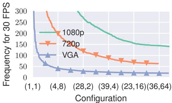
Figure 8: Frequency needed to achieve 30 frames per second on the proposed architecture for varying degrees of parallelism.
