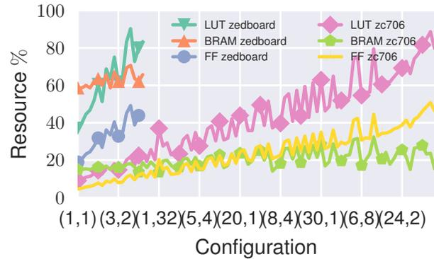
Figure 9: Hardware synthesis results for accelerators at VGA resolution for Zedboard and ZC706 platforms
