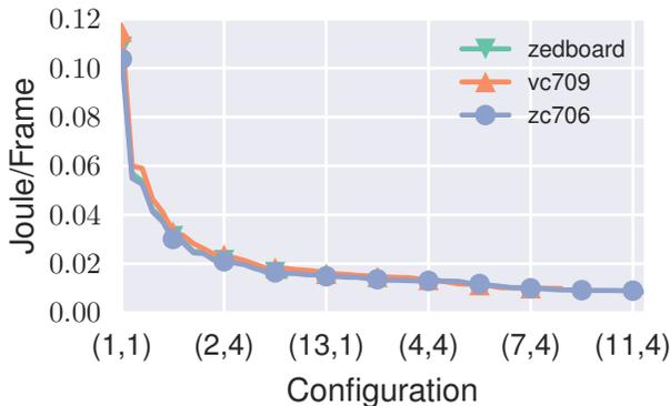
Figure 12: Energy consumed by different configurations of VGA-resolution SGM accelerators at maximum fps
