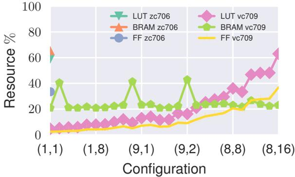
Figure 11: Hardware synthesis results for accelerators at 1080p resolution for ZC706 and VC709 platforms
