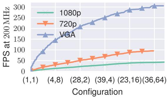
Figure 7: Frames per second achieved by the proposed architecture at a clock frequency of 200 MHz.
