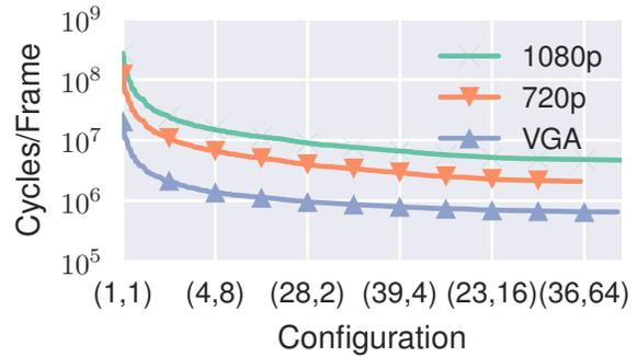
Figure 6: Cycles needed to process a single disparity map for varying degrees of parallelism.
