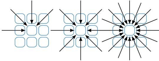
Figure 2: (a) Four, (b) Eight, and (c) 16 directions used in Semi-Global Block Matching.
