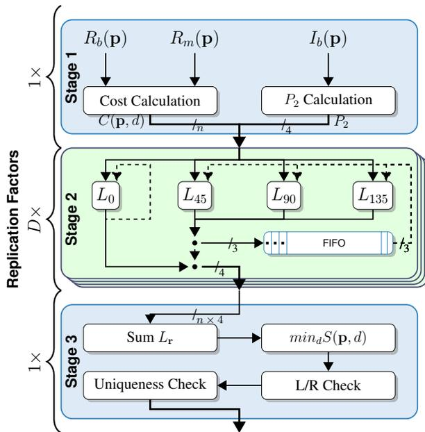
Figure 4: Extending the base architecture with fine-grained parallelism: Parallel cost computations (per-pixel, per-path) for multiple potential disparity values
