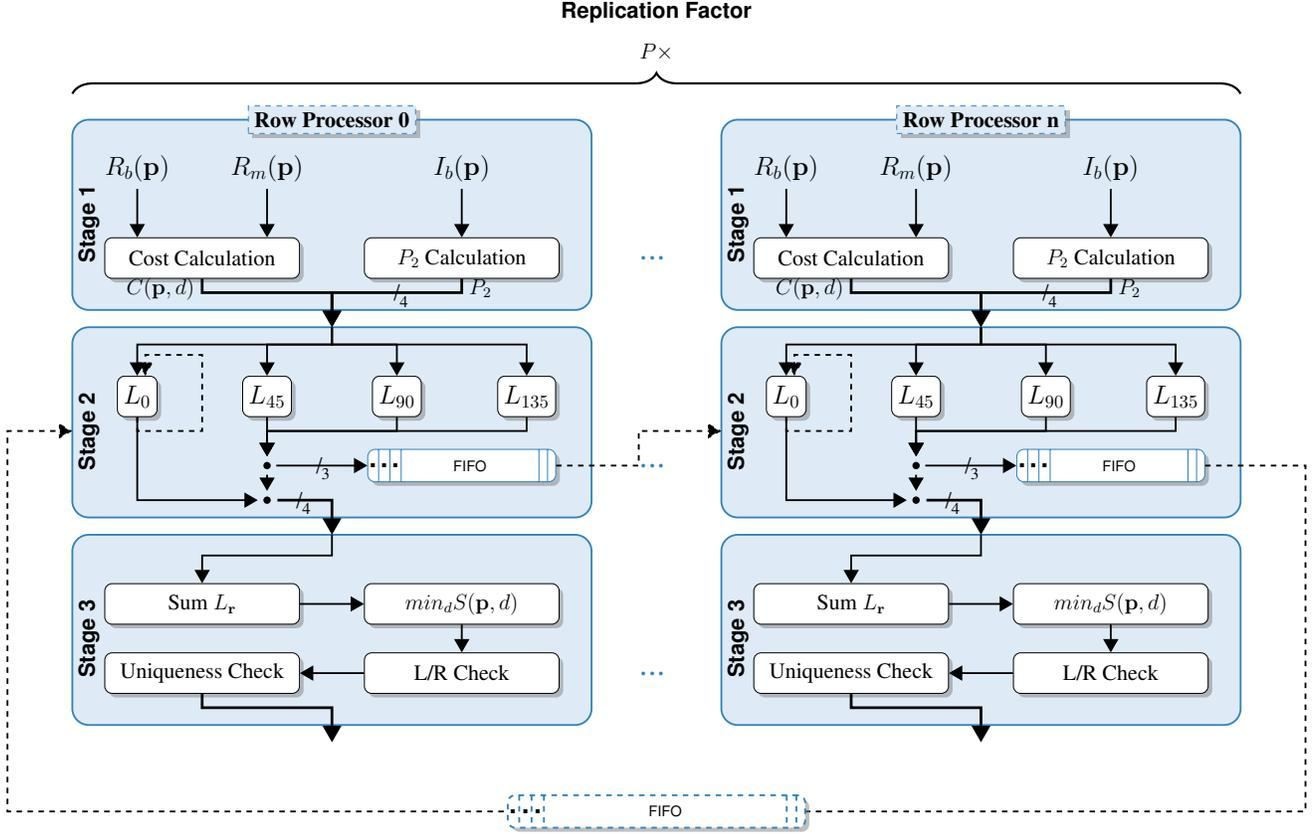
Figure 5: Coarse-grained parallelization: Processing multiple rows in parallel
