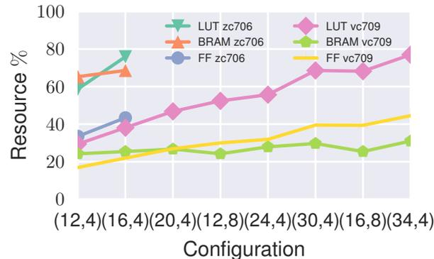
Figure 10: Hardware synthesis results for accelerators at 720p resolution for ZC706 and VC709 platforms
