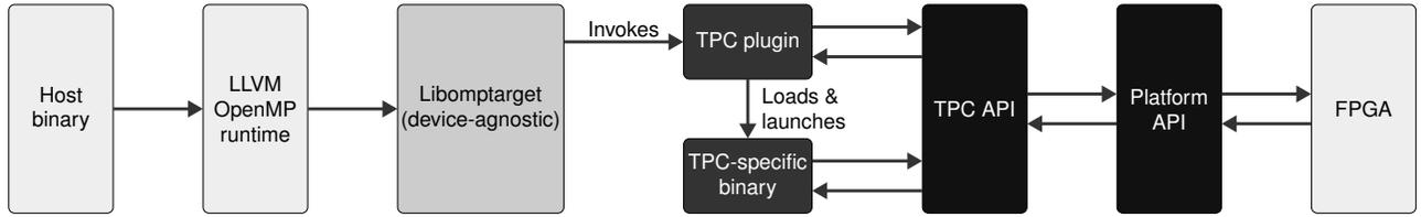
Fig. 2. Runtime flow for TPC FPGA offloading.
