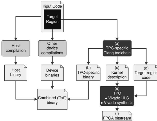
Fig. 1. Custom device toolflow for Clang.
