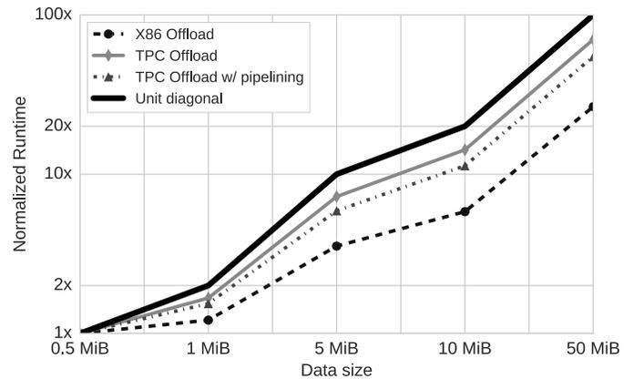
Fig. 4. Normalized runtime vs. data size in the *vector scaling* benchmark.
