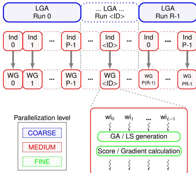
Figure 3: Visualization of AutoDock-GPU computations being mapped onto OpenCL elements. Basically, a population processed by an LGA run ( $Run_{ID}$ ) is decomposed into their individuals, and each individual ( $Ind_{ID}$ ) is mapped onto a work-group ( $WG_{ID}$ ). Fine-grained tasks are processed by work-items ( $wi_0 \dots wi_{L-1}$ ).
