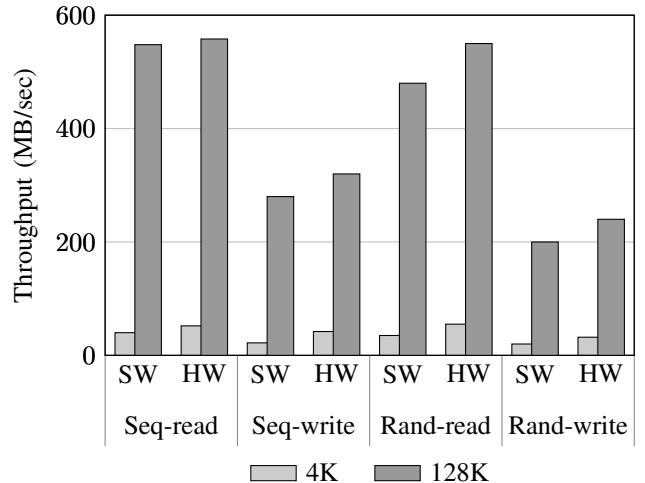
Fig. 4: Block I/O Throughput Hardware-Accelerated vs Software Baseline
