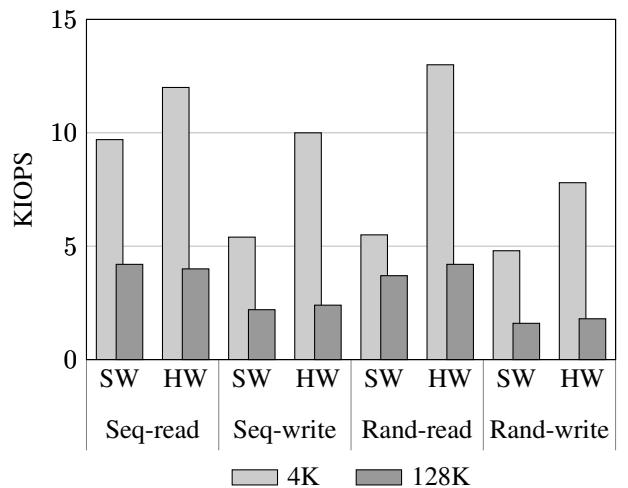
Fig. 5: IOPS on Hardware-Accelerated Stack vs Software Baseline
