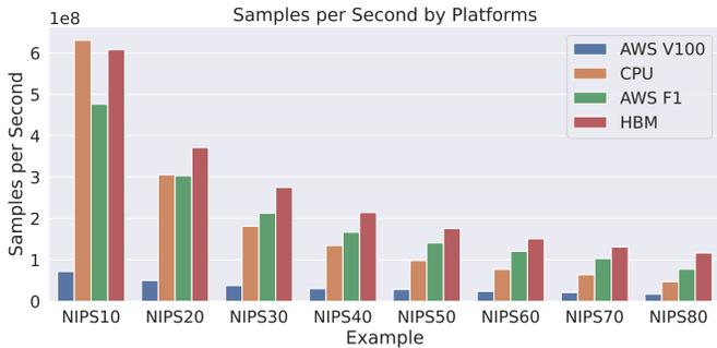
Fig. 6. Peak performance measurements for the different benchmark SPNs on different target platforms. The number of samples per second is calculated from the end-to-end execution time. For AWS F1, V100 and HBM, host-to-device data transfers are *included* in the runtime.
