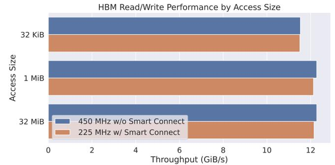
Fig. 2. Maximum throughput when issuing linear read and write accesses in parallel to one HBM memory channel for two different configurations and different request sizes. The first configuration runs the block generating the accesses with the 450 MHz clock used by the HBM and natively connects both. The second configuration runs the PE at *half* the clock frequency but the interface width is *doubled*. An AXI Smart Connect is used to perform clock- and data-width-conversion.
