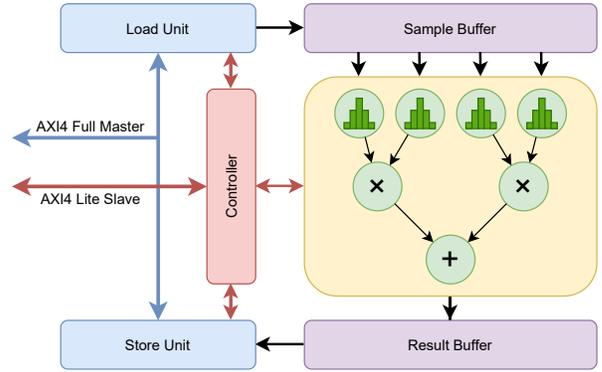
Fig. 3. Architecture of the SPN-Accelerator
