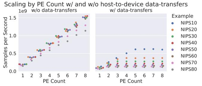
Fig. 4. Comparison of peak performance in samples per second. On the left, host-to-device data-transfers are excluded to disregard a PCIe-based bottleneck. On the right, actual end-to-end performance is measured. Note that the inclusion of the data-transfer time leads to severely skewed scaling.
